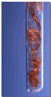
Figure 16.2.1: Reaction of copper wire in a silver nitrate solution.
